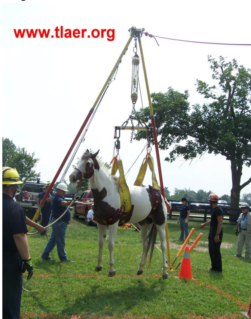
The Becker Sling lifting a horse under an A Frame
